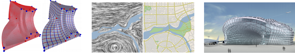
Figure 4.3: New applications emerging from recent orientation field modeling methods: (from left to right) mixed-integer quadrangulation [6], procedural city design [10], and planar quad mesh design useful for architectural glass structures [61].
