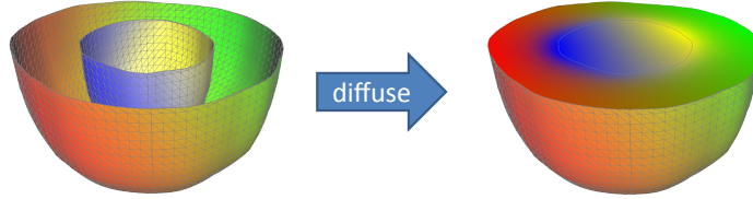
Figure 6.2: The concept of the DSs representation. A set of colored surfaces (left) defines a volumetric color distribution (right) by diffusing colors in 3D space.
